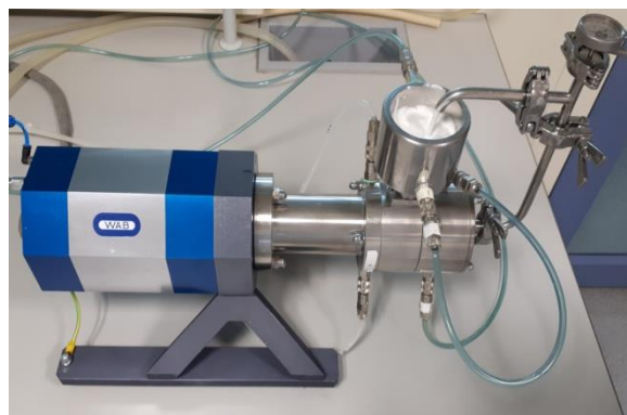
Slika 10. Mlin Dyno-mill Research Lab ( WAB, Švicarska )
