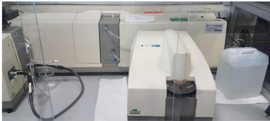
*Slika 3.5 Malvern Instruments MS2000 PSD instrument*
