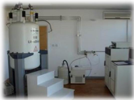
**Slika 14.**  $^1\text{H}$  NMR spektrometar *Bruker Avance 300* (CIL, INA d.d.)
