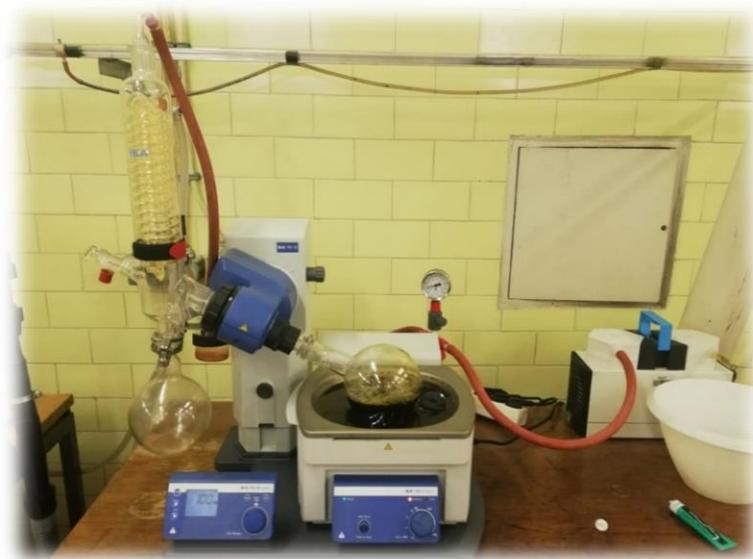
**Slika 10.** Vakuum isparivač IKA RV 10, *rotary evaporator, basic*
