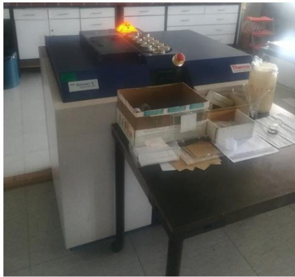
Slika 26. Valno-disperzivni X-ray spektrometar ARL ADVANT'X+ Sequential XRF,
