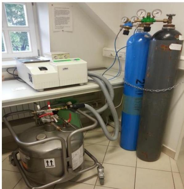
**Slika 12. DSC instrument Mettler Toledo DSC 822e**
