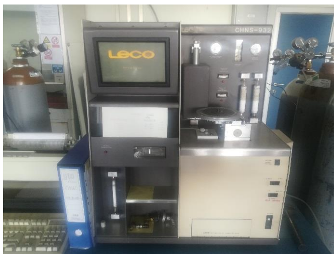
Slika 19. Leco CHN 628 Carbon/Hydrogen/Nitrogen Determinator
