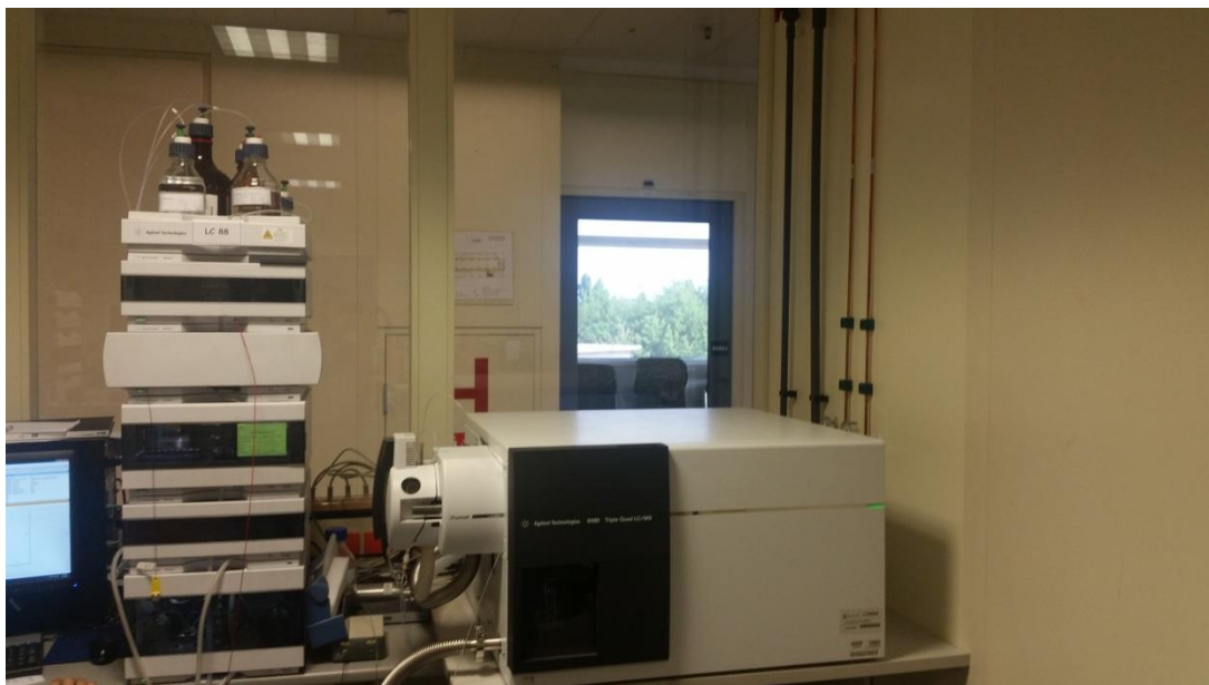
Slika 3.2.5. UHPLC Agilent Series 1290
