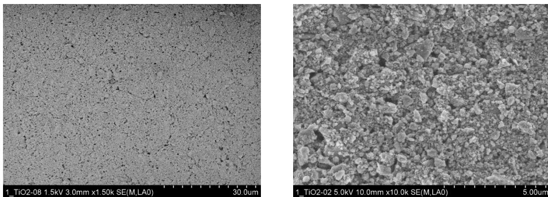
Slika 11. SEM slike prevlake A  $\text{TiO}_2 + 1 \text{ at.\% Sm}$
