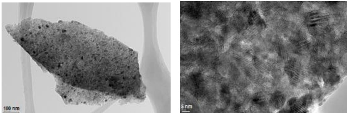
Slika 7. HRTEM slike praha A  $\text{TiO}_2 + 1 \text{ at.\% Sm}$
