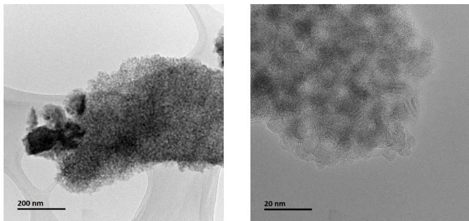
Slika 9. HRTEM slike praha E  $\text{TiO}_2 + 1 \text{ at.\% Nd}$
