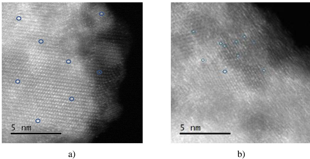
Slika 10. HAADF-TEM slike a) praha A  $\text{TiO}_2 + 1 \text{ at.\% Sm}$ , b) praha E  $\text{TiO}_2 + 1 \text{ at.\% Nd}$
