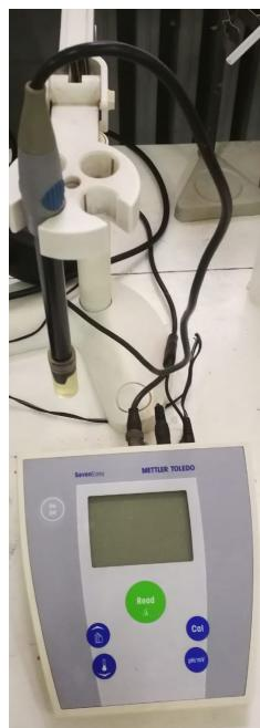
**Slika 16 - pH - metar Mettler Toledo**
