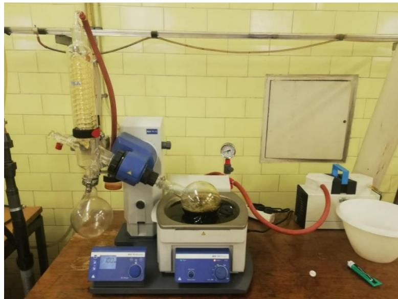
**Slika 13.** Vakuum isparivač IKA RV 10, *rotary evaporator, basic*
