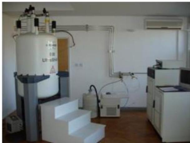
Slika 23.  $^1\text{H NMR}$  Spektrometar *Bruker Avance 300* (CIL, INA d.d.)
