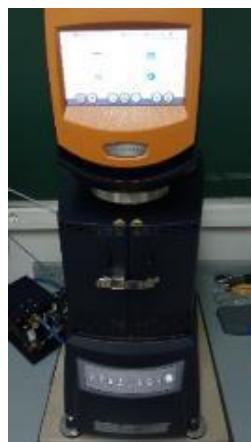
Slika 3.5 Reometar Discovery HR 30
