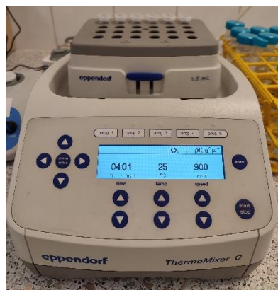
Slika 3.2. Termostatirana tresilica Eppendorf ThermoMixer C
