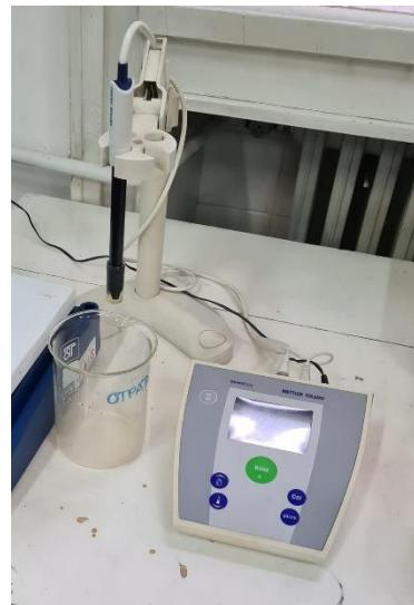
Slika 8. pH metar Mettler Toledo S20 SevenEasy
