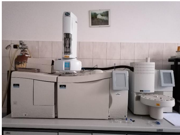
Slika 4. GC/MS instrument Clarus 500
