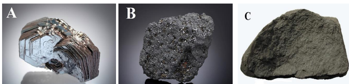
Slika 3. Kristali hematita (A) [6], magnetita (B) [7], i maghemita (C) [8].
