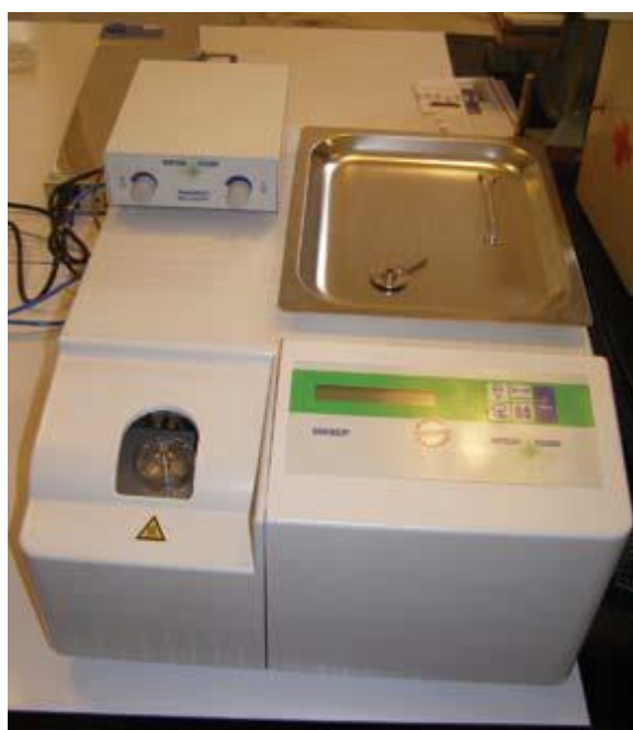
Slika 3.7. Mettler Toledo DSC823 e , ZIPPM, FKIT 23
