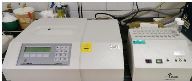
**Slika 3.16.** Luminometar LUMIStox 300 i termometar LUMIStherm, Hach-Lange GmbH.
