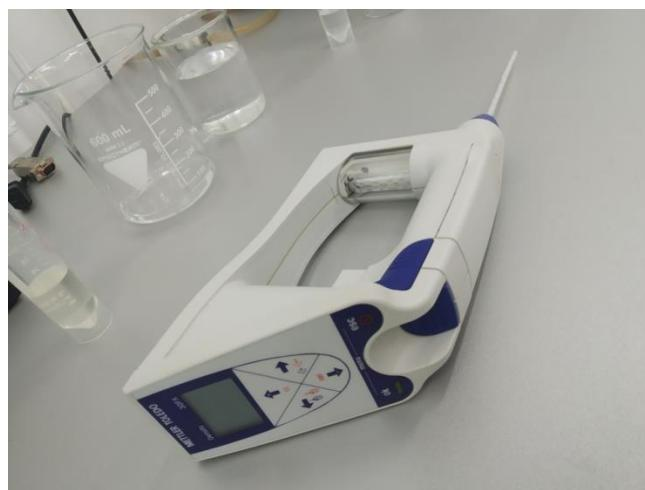
**Slika 8.** *Mettler toledo densitometer 30PX.*
