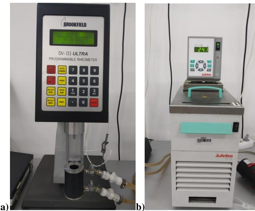
**Slika 7.** a) Reometar *Brookfield DV-III ULTRA*, b) Termostat *Julabo F12*
