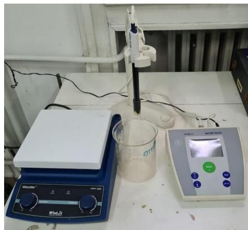
Slika 3.3. pH-metar *Mettler Toledo, S 20 SevenEasy*
