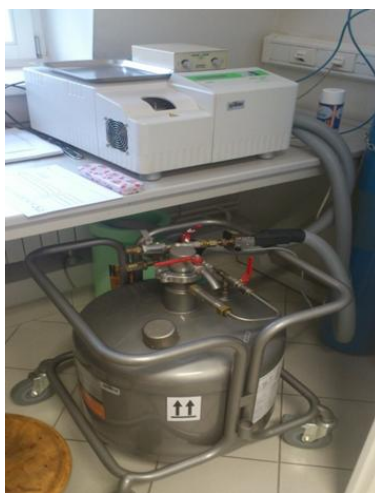
Slika 10. DSC instrument Mettler Toledo DSC 822 e
