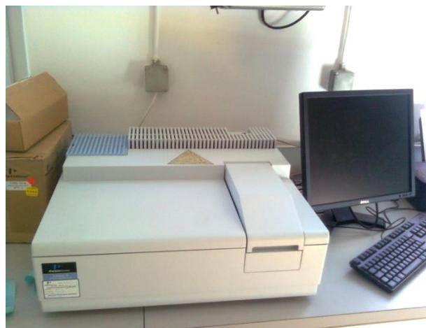
*Slika 3.26. UV/VIS spektrofotometar Lambda 35 (PerkinElmer, Waltham, SAD)* <sup>[22]</sup>
