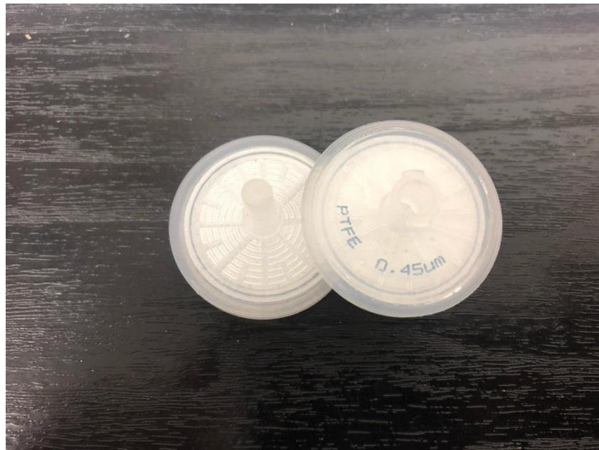
Slika 3.15. PTFE (*Polytetrafluoroethylene*) filteri
