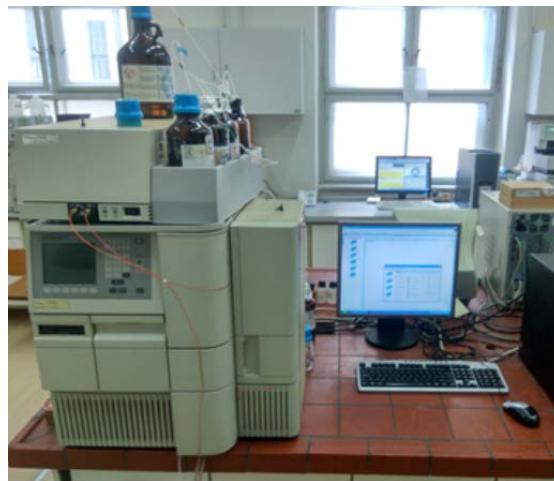
**Slika 25.** Waters 2795 Alliance HPLC sustav s 2996 PDA detektorm
