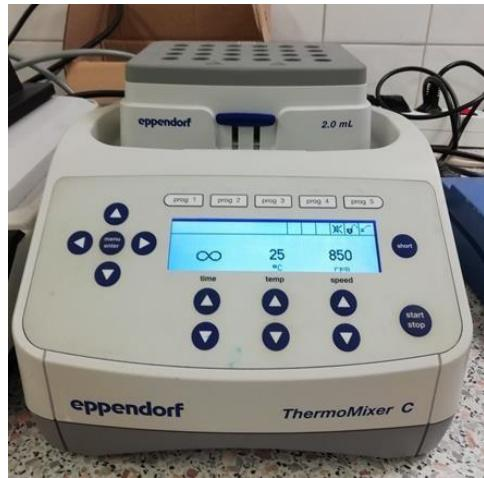
**Slika 12.** Termostatirana tresilica Eppendorf ThermoMixer C
