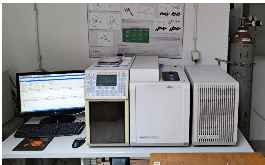
Slika 12. GC-MS sustav Varian CP 3800-Varian Saturn 2200
