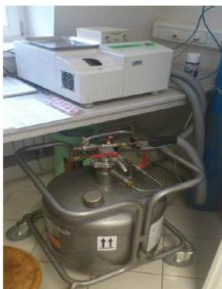
**Slika 26.** DSC analizator Mettler Toledo 822<sup>e</sup>
