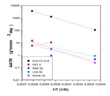
Figure 5.11. Arrhenius plot "AATR vs. reverse temperature" for PET monolayers
