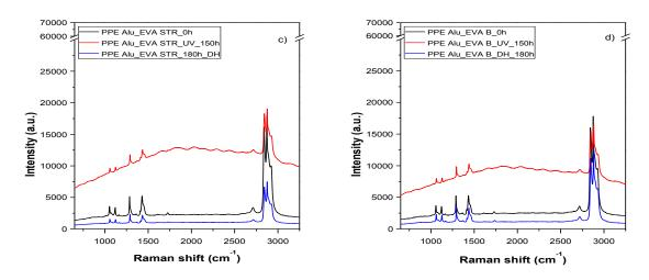
**Figure 5.18.** Raman spectra of the laminates with encapsulation after different aging conditions: a) AAA/EVA STR; b) AAA/EVA BRIDGESTONE; c) APA/EVA STR; d) APA/EVA BRIDGESTONE; e) PPE/EVA STR; f) PPE/EVA BRIDGESTONE; h) PPE Alu/EVA STR; i) PPE Alu/EVA BRIDGESTONE
