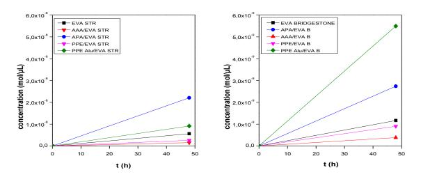
**Figure 5.12.** Concentration of acetic acid formed within 48 h of exposure to UV/T in EVA STR (left) and EVA Bridgestone (right)
