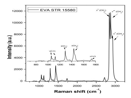
Figure 5.16. Raman spectrum of an unaged EVA minimodule
