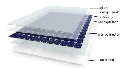
Figure 2.3. Design of photovoltaic module [11]
