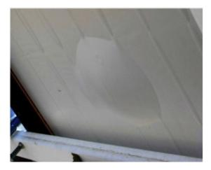
Figure 2.7. Delamination of backsheet [11]
