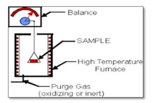
**Figure 3.1.** Schematic of TG analyzer [53]
