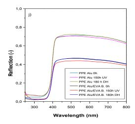
**Figure 5.15.** Spectra of unaged and aged minimodules and backsheets:a) EVA STR, b) EVA BRIDGESTONE, c) AAA/EVA STR; d) AAA/EVA BRIDGESTONE; e) APA/EVA STR; f) APA/EVA BRIDGESTONE; g) PPE/EVA STR; h) PPE/EVA BRIDGESTONE; i) PPE Alu/EVA STR; j) PPE Alu/EVA BRIDGESTONE
