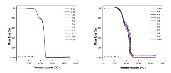
**Figure 5.4.** TGA curve for dynamical measurements of EVA STR 15580 in inert (left) and oxidative atmosphere (right)
