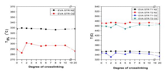
**Figure 5.5.** Influence of degree of crosslinking on value of  $T_{5\%}$  (left) and  $T_{1max}$  and  $T_{2max}$  (right) in inert and oxidative atmosphere
