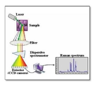
Figure 3.5. Schematic of Raman spectroscopy [63]
