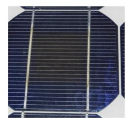
**Figure 2.6.** Slightly browned EVA in the center of a multicrystalline Si-cell [11] Delamination can occur between the boundary surfaces of glass to encapsulant, encapsulant to solar cell, encapsulant to backsheet and within the layers of the backsheet (Figure 2.7.) [34,37]
