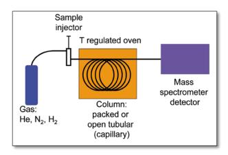
Figure 3.3. Schematic of GC-MS [57]
