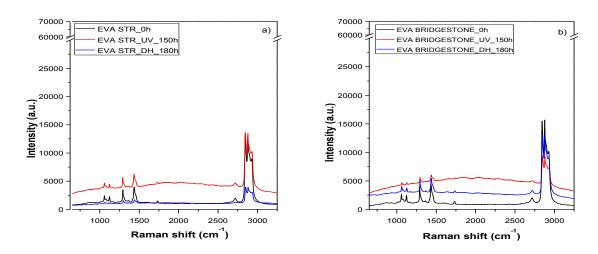
**Figure 5.17.** Raman spectra of unaged and aged EVA STR minimodules (a), and EVA BRIDGESTONE (b) after UV and DH exposure
