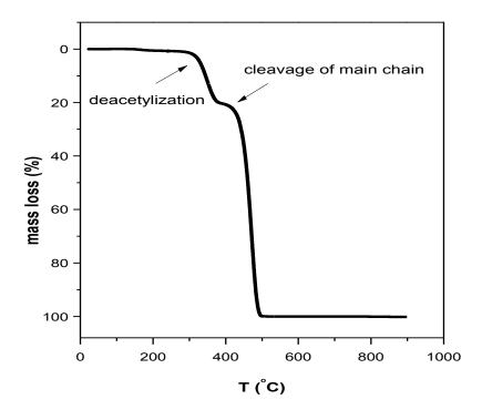
Figure 5.1. Typical TGA curve of EVA
