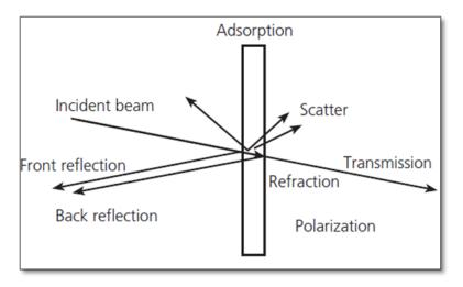
**Figure 3.4**. Interactions of light with solid sample [58]
