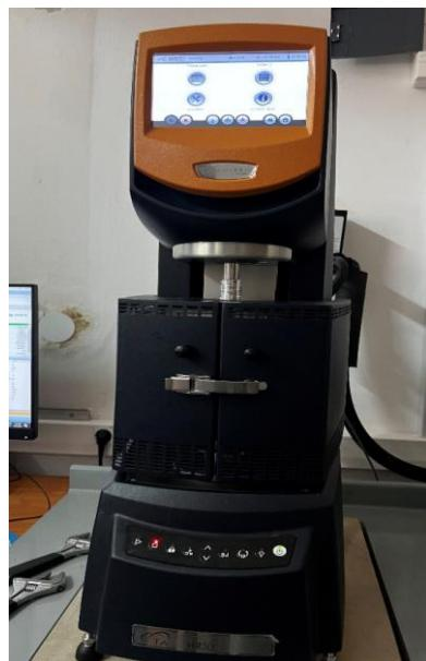
**Slika 39.** Reometar HR 30, TA Instruments
