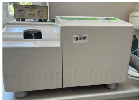
**Slika 14.** DSC instrument Mettler Toledo DSC 82
