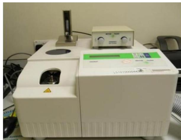
*Slika 22.* Mettler Toledo DSC 823eT kalorimetar
