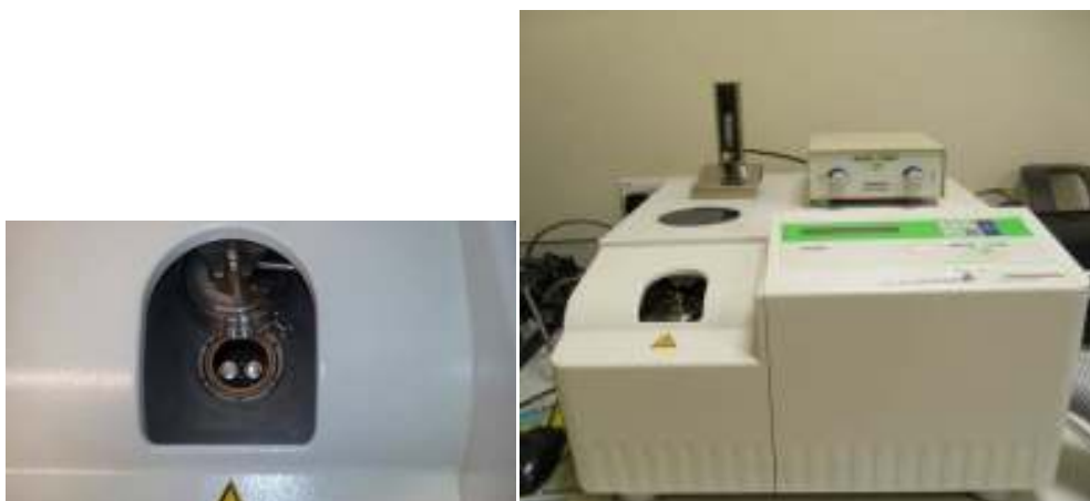
Slika 18. DSC instrument Mettler Toledo DSC 822 e .
