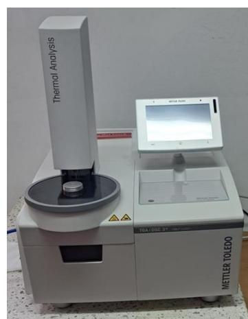
Slika 2.13. TGA analizator, TGA/DSC 3+ Mettler Toledo
