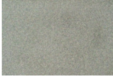
Figure 32: The panel prepared by the surface preparation method Sa 2.5
