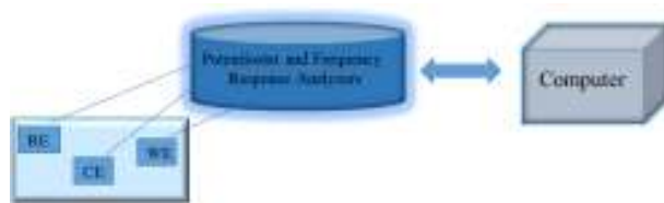
Figure 36: Scheme of electrochemical impedance spectroscopy (EIS) measurements
