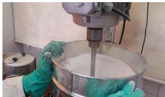
Figure 30: Mixing all ingredients of the coating in the final step
