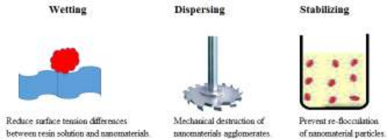
Figure 13: The dispersion of nanoparticles in liquid matrices
