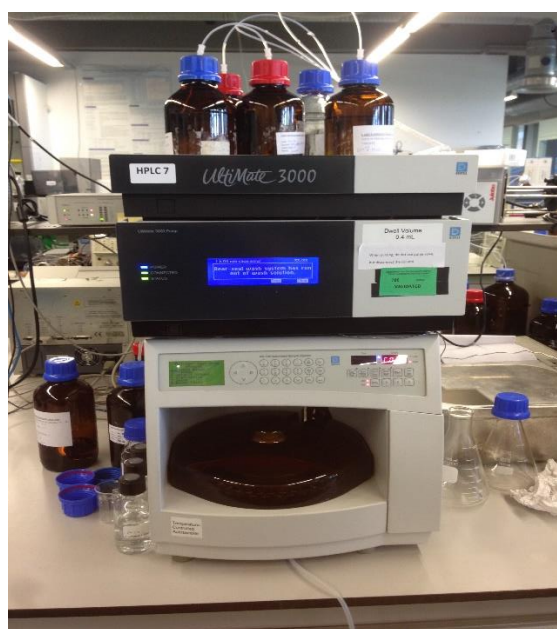
Figure 6 Dionex pump and autosampler
