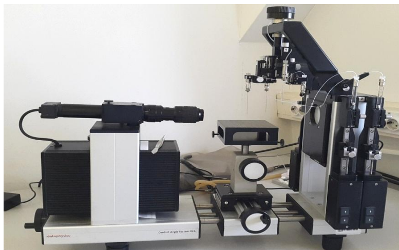
Slika33. Goniometar DataPhysics OCA 20 Instruments, GmbH
