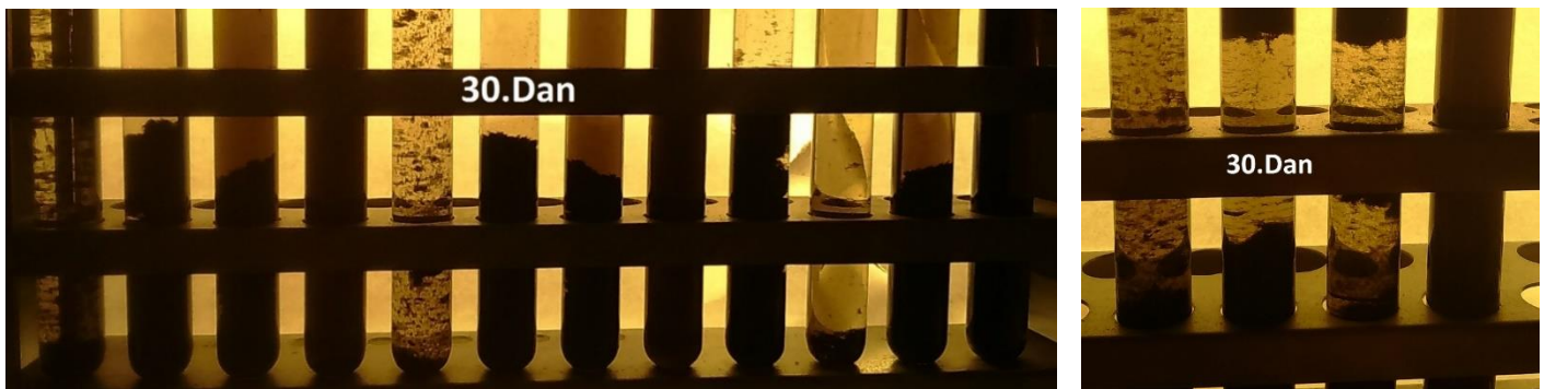
Slika 4.2.14. Sedimentacijski test nanofluida (s lijeva na desno: PDPA, PDPA2, PDPA5, PDPA10, PDPS, PDPS2, PDPS5, PDPS10, YDPA, YDPA2, YDPA5, YDPA10, YDPS, YDPS2, YDPS5, YDPS10), 30. dan
