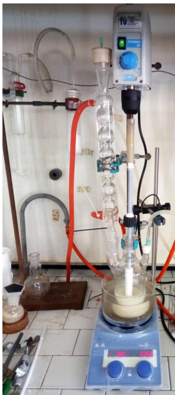
Figure 27. Suspension polymerization reactor used in laboratory
