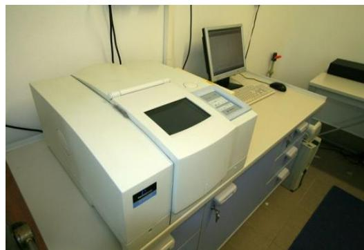
**Slika 3.2.** Perkin Elmer Spectrum One FTIR spektrometar
