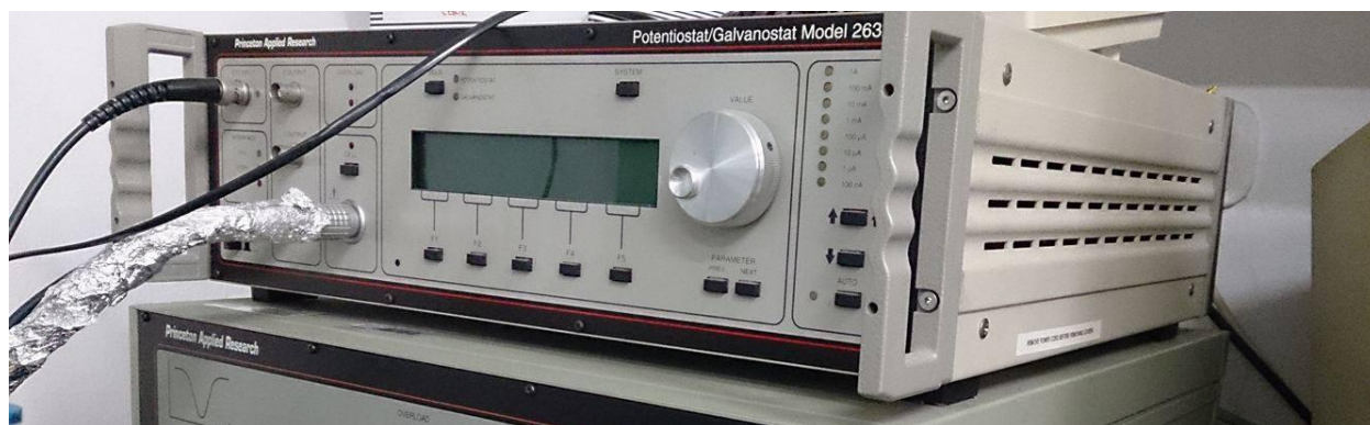
Slika 3.8. Potenciostat: EG&G Princeton Applied Research, model 263A
