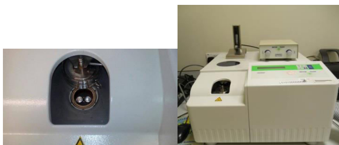
Slika 13. DSC instrument Mettler Toledo DSC 822 e
