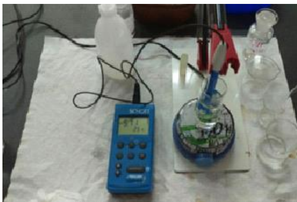
Slika 10. Prenosivi pH metar, Handylab pH/LF, Schott Instruments GmbH
