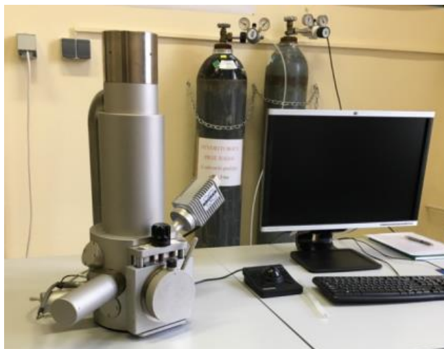
Slika 23. Tescan Vega 3 SEM, neparivač (sputtercoater) Quorum SC7620
