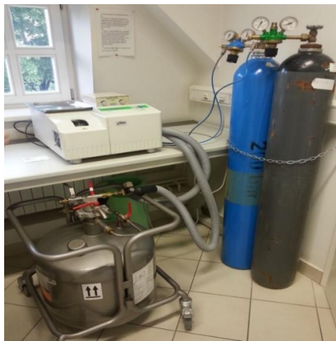
Slika 15. DSC instrument Mettler Toledo DSC 822 e .
