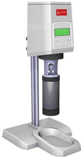
**Slika 22.** Reometar Auton Paar Rheolab QC
