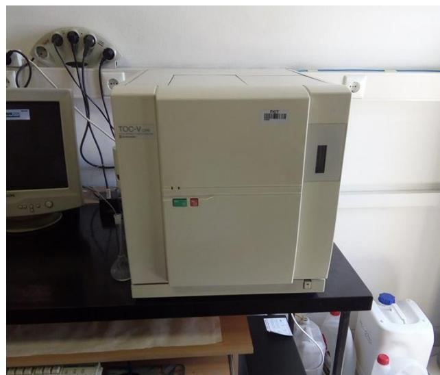
**Slika 9.** TOC-VCPN Total Organic Carbon Analyzer, Shimadzu.
