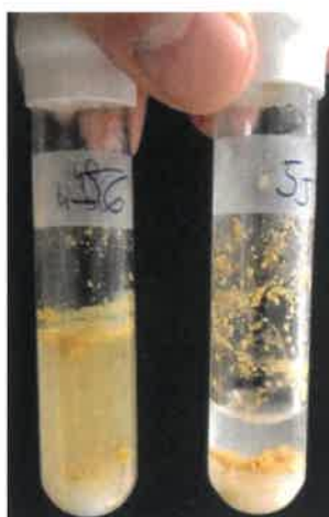
Figure 16 The resulting mixtures of 0.1 M (left) and 0.2 M (right) concentrations with a solvent ratio of 1:1 with K_2HPO_4 as base.
