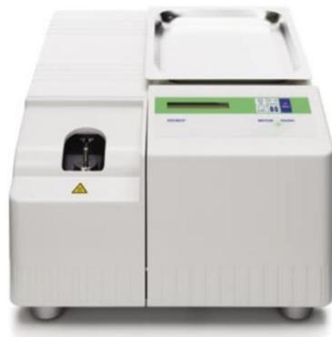
**Slika 21.** DSC Mettler Toledo 823<sup>e</sup>
