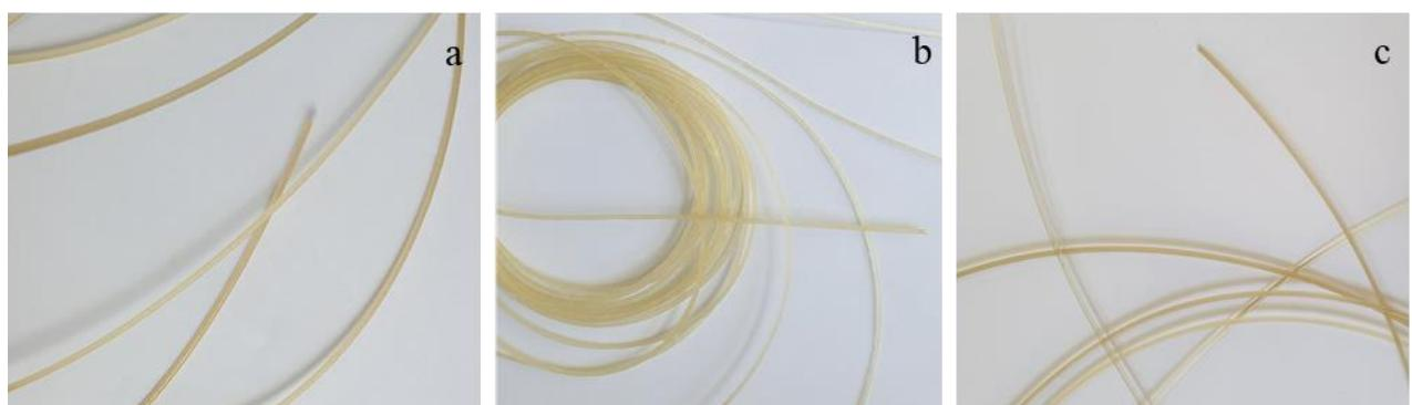
**Slika 18.** Dobiveni filamenti: a) PVA FF 10% 150, b) PVA FF 10% 160, c) PVA FF 10% 170
