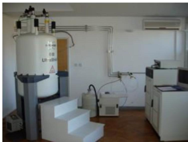
Slika 3.8:<sup>1</sup>H NMR Spektrometar Bruker Avance 300
