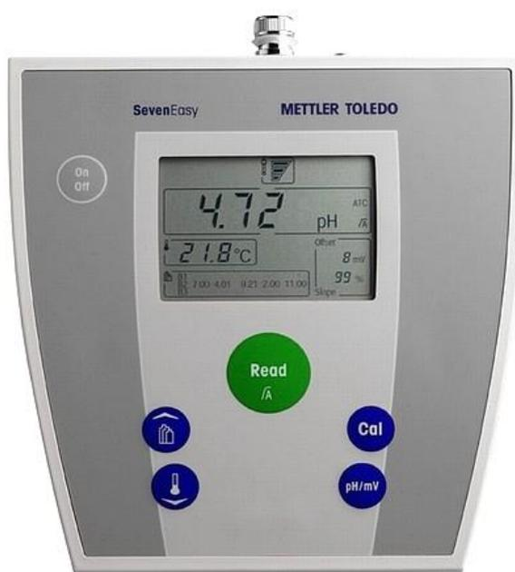
Slika 8. pH-metar Mettler Toledo S20 SevenEasy
